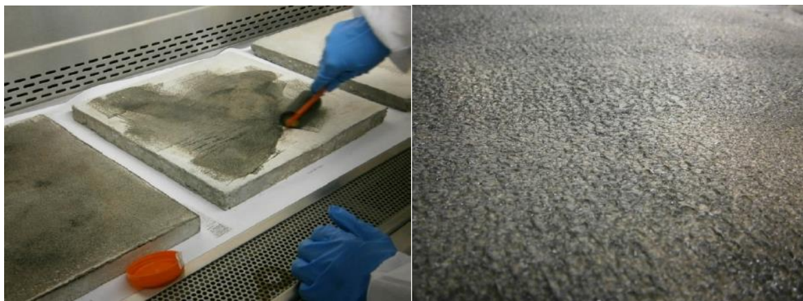
Figure 1. Photo of Model Agricultural Grime Application to Concrete Test Coupons.
