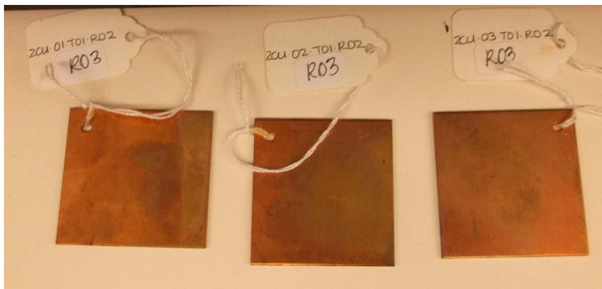
Figure 3-2. Copper exposed to EtO (2Cu-01 and 2Cu-02 on left) and not exposed (2Cu-03 on right)
