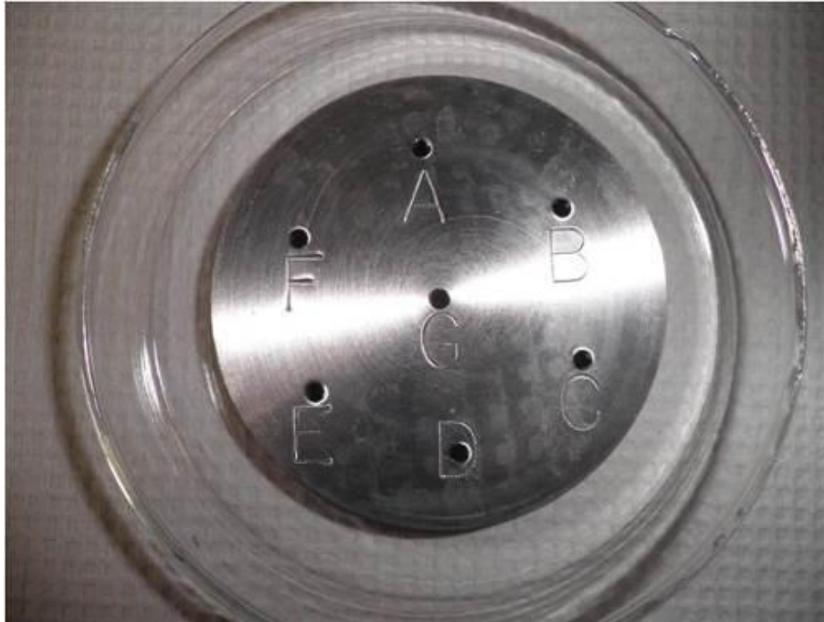
Figure 2-5. 18-mm Stub Stage in Container
