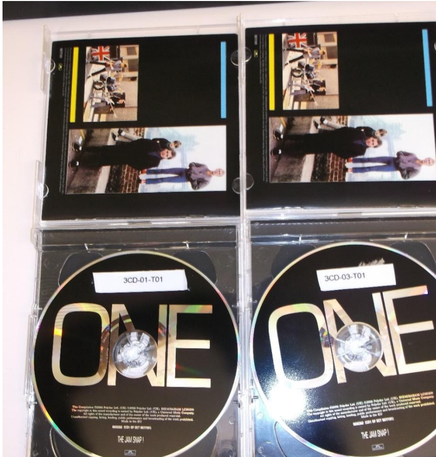
Figure 3-10. Exposed (left) and unexposed (right) CD 10 months later
