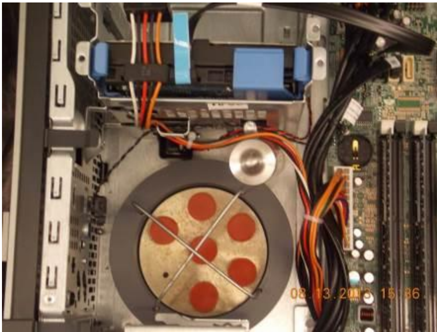
Figure 2-6. Location of MadgeTech device and rubber coupons within the computers (between the CD drives and hard drives)
