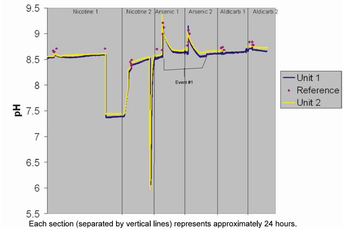
**Figure 6-4. Stage 2 Contaminant Injection Results for pH**
