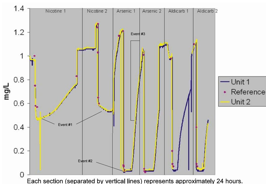
**Figure 6-1. Stage 2 Contaminant Injection Results for Total Chlorine**
