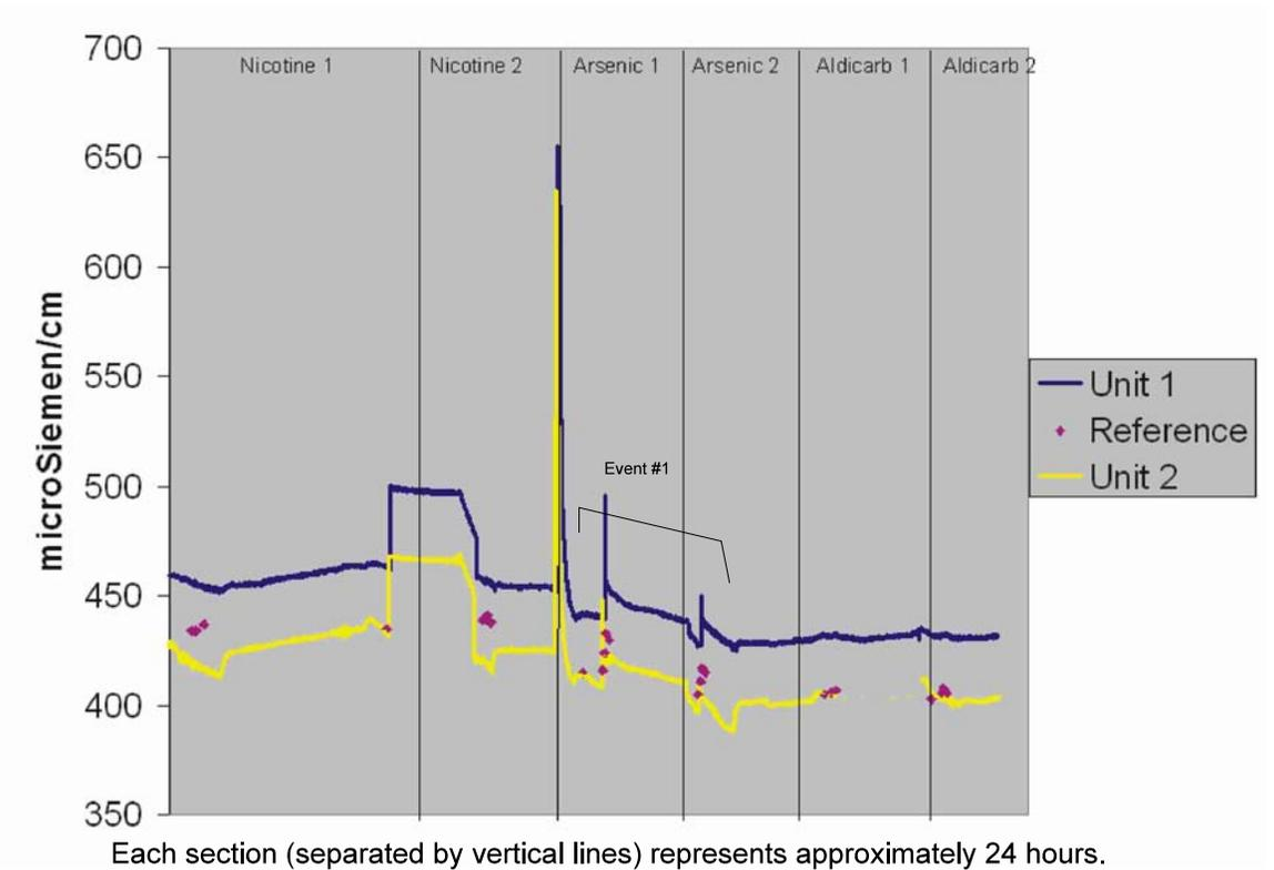
**Figure 6-5. Stage 2 Contaminant Injection Results for Conductivity**
