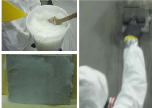
Figure 5-1. ASG in container prior to application (top left), after application to concrete coupon (bottom left), and during vacuum removal (right).
