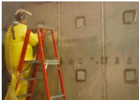
**Figure 3-2. Containment tent: outer (left) and inner view with test stand containing contaminated coupons (right).**
