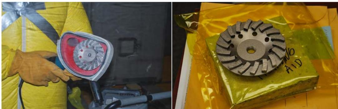
**Figure 2-1. Angle grinder equipped with SDG and DMD (left). DMD (right).**
