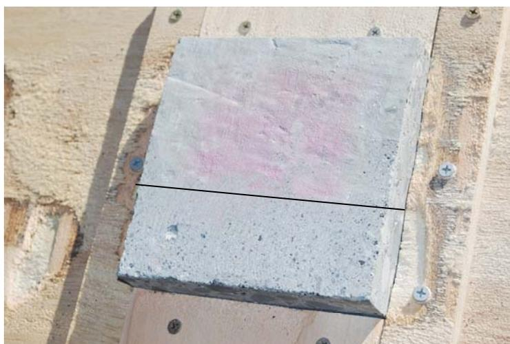
**Figure 5-1. Concrete coupon demonstrating surface damage.**
