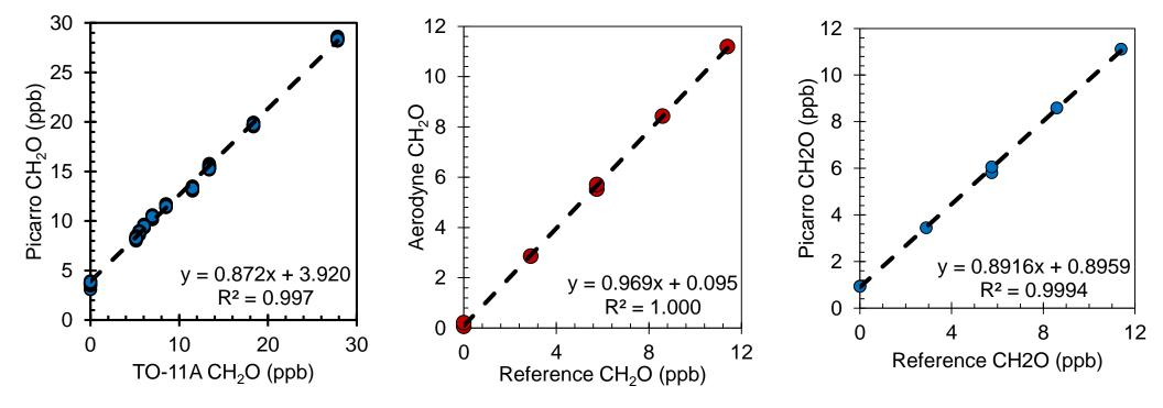
Picarro and Aerodyne compare well to reference formaldehyde from permeation tubes (left) and gas cylinders (center, right).
