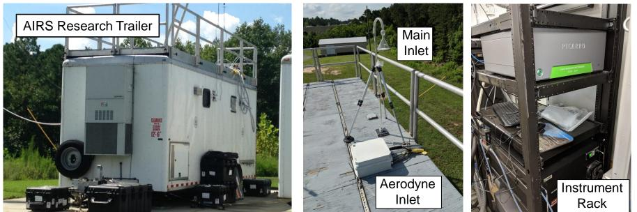
Between June 2018 and July 2018, we ran the Aerodyne (for one week), Picarro, and Gasera formaldehyde monitors in a research trailer at the Ambient Air Innovative Research Site (AIRS) in Research Triangle Park, NC. We also ran collocated DNPH cartridges for several periods.
