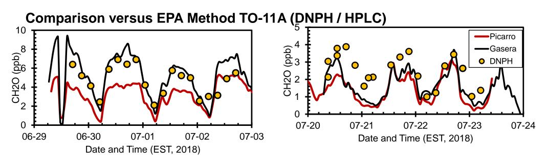
Comparison between spectroscopic measurements (Aerodyne, Gasera, and Picarro) and EPA Method TO-11A measurements do not always agree. Spectroscopic CH<sub>2</sub>O was lower than TO-11A CH<sub>2</sub>O during tests at both Research Triangle Park, NC and Flax Pond (New York, data not shown) sites. This source of these discrepancies in unclear and is currently under investigation.
