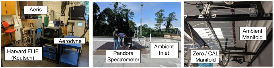
Between September 2018 and October 2018, we ran the Aerodyne and Picarro instruments collocated at the Flax Pond Marine Laboratory in Old Field, NY as part of the Long Island Sound Tropospheric Ozone Study (LISTOS). Harvard University ran a fiber laser induced fluorescence instrument and Aeris formaldehyde monitor, SUNY Stony Brook ran a PTR-MS, and the New York DEC ran PAMS-style DNPH cartridges. The Gasera instrument was also run towards the end of the study.
