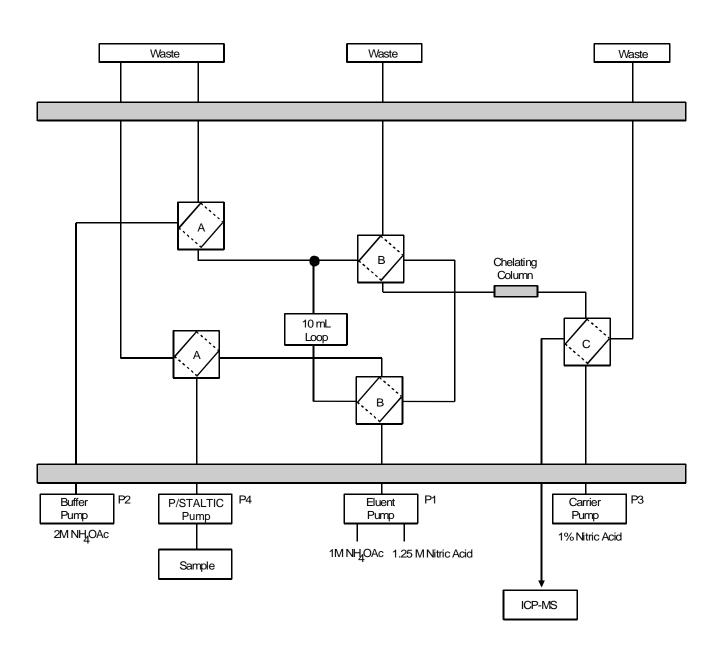
Figure 1. Configuration of Preconcentration System.
