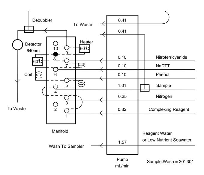
Figure 1. Manifold Configuration for Ammonia Analysis.
