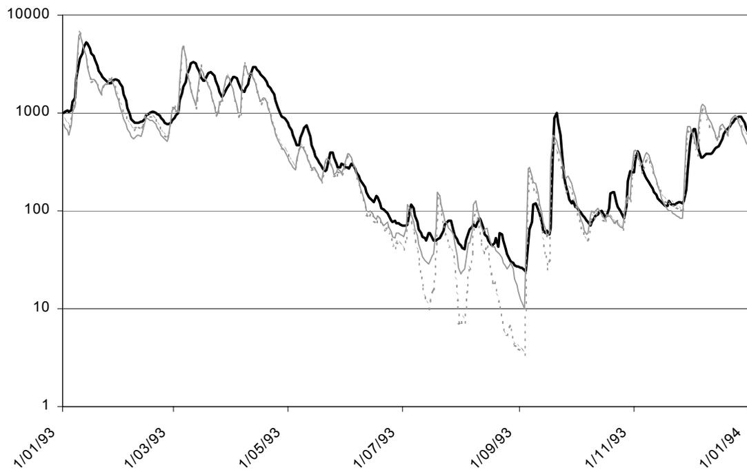
Figure 29a. Model-generated (light lines) and measured (bold line) flows in  $\text{ft}^3/\text{sec}$  over 1993. Model parameters were estimated using PEST's predictive analysis functionality.
