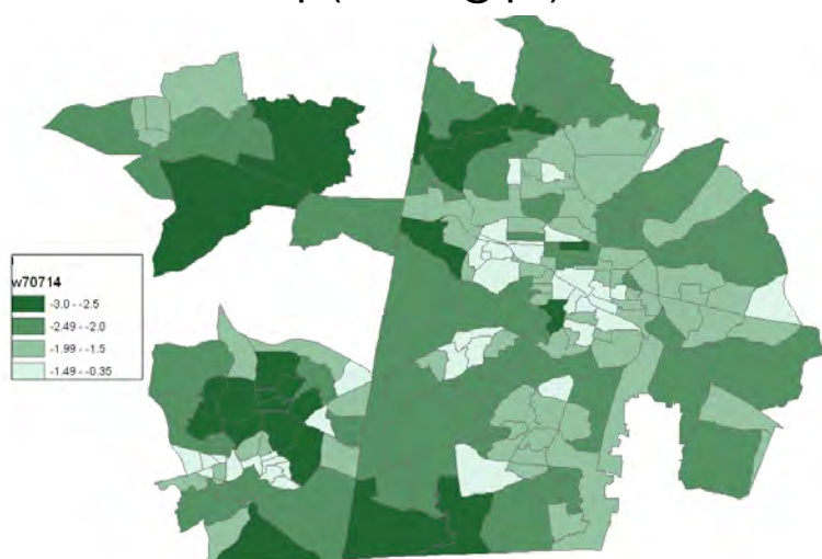
Reduc. ambient temp. (07/07/10 @2pm) due to tree cover
