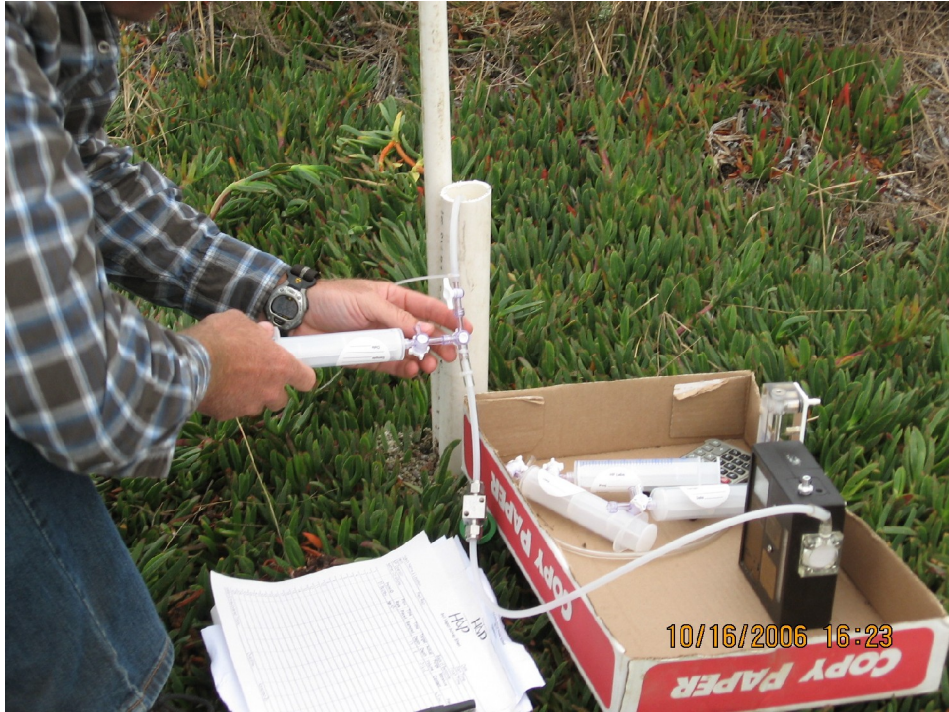
Photograph 9 – Sampling using battery operated pump to purge and 60 ml syringe for sample collection.
