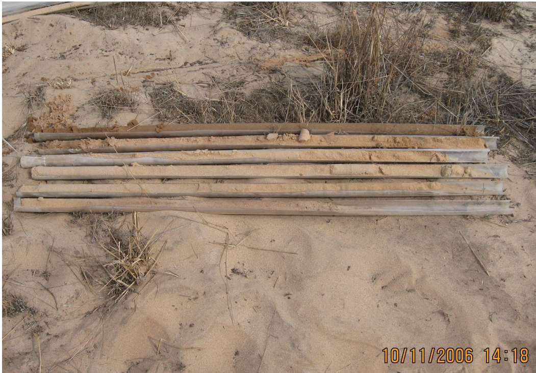
Photograph 5 – Soil cores from 15-SV-A1. Soils increase in depth from right to left and from bottom to top of field of view. Each acetate sleeve is 4 feet long. Soils from greater depths are darker due to higher moisture content; soil type and composition is homogeneous throughout borehole.
