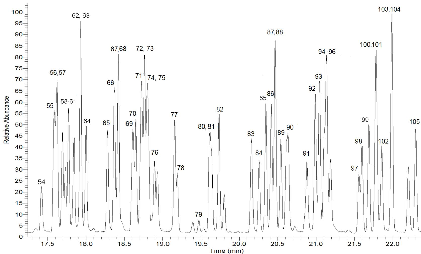
**Figure 1d. Example chromatogram of a calibration standard (concentration of 5 ng/ $\mu$ L injected for most analytes). Peak identification numbers correspond to those in Table 1.**
