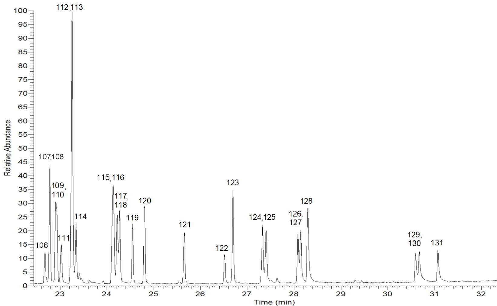
**Figure 2. Example extracted ion current profiles of toxaphene at m/z 125, 305, and 159.**
