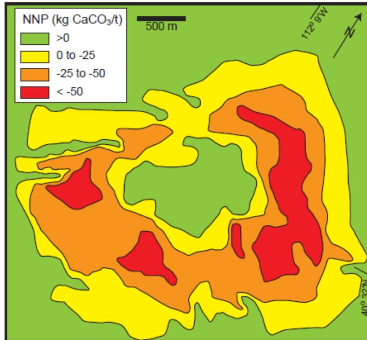
**Figure 6.** Plan view of the distribution of net neutralizing potential (NNP) values at the Bingham Canyon porphyry copper deposit, Utah. NNP values above zero are “net alkaline”; those below zero are “net acid”. Modified from Borden (2003).
