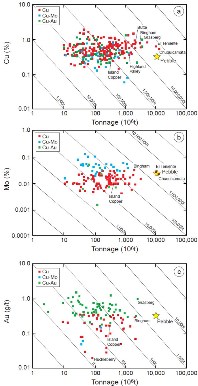
**Figure 4.** Grade-tonnage characteristics of the Pebble deposit compared to other porphyry-type deposits. A. Copper; B. Molybdenum; C. Gold. The Pebble deposit is shown as the yellow star. Selected, noteworthy deposits are labeled. Pebble is classified as a porphyry Cu deposit (red squares). The dashed diagonal lines represent the total contained metal. Modified from Sinclair (2007).
