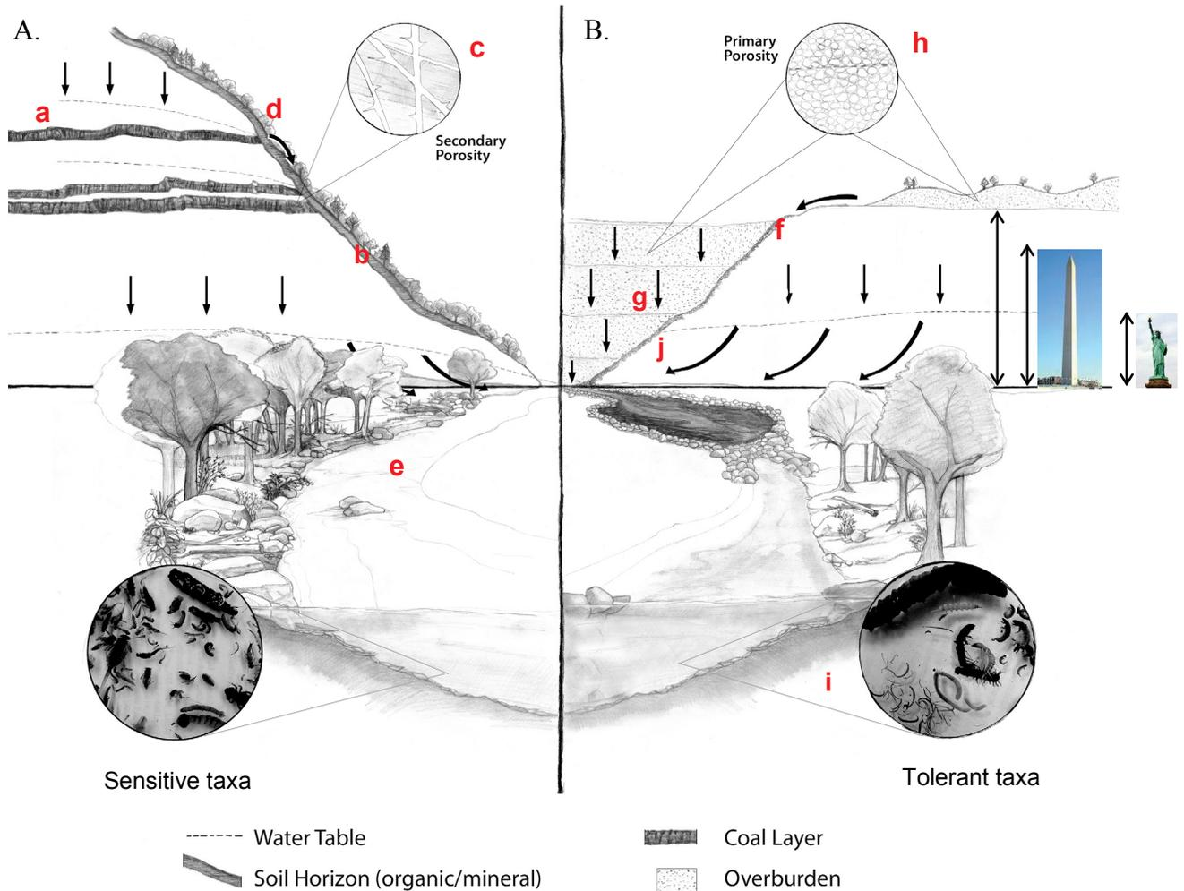
**Figure 5. Small stream watershed before and after mountaintop mining and creation of a valley fill (simplified view).** Monuments added for scale. Scales differ between upper and lower halves of diagram.
