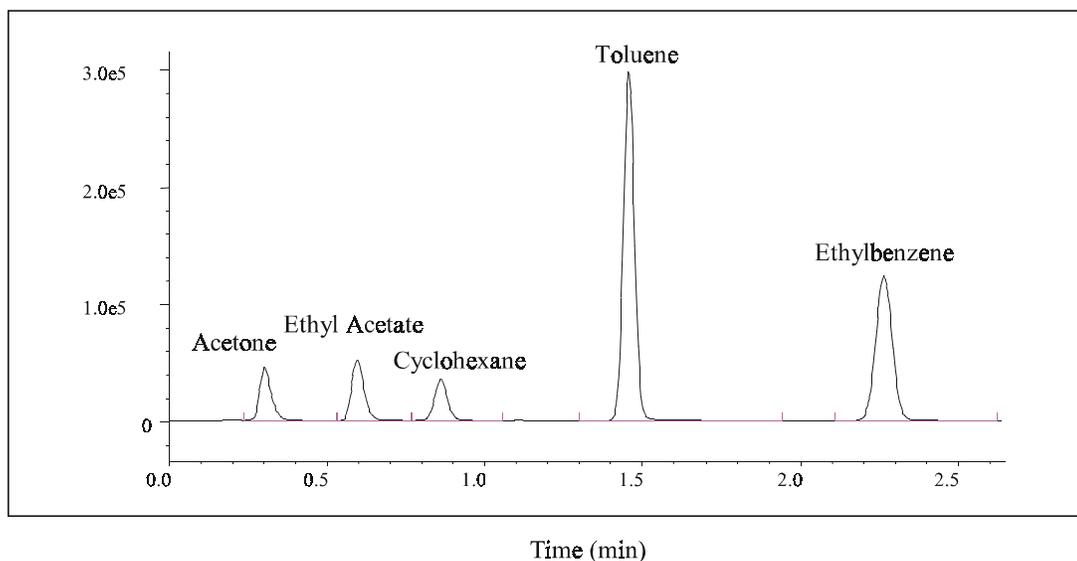
**Figure 3-2. Liquid-phase sample chromatogram.**
