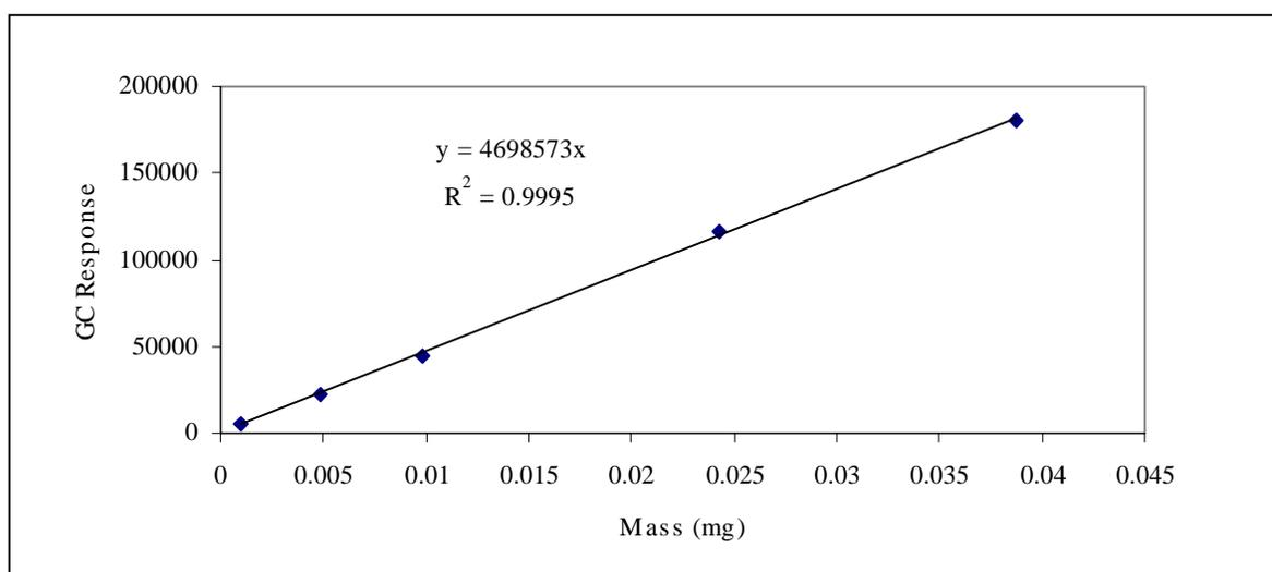
**Figure 3-5. Gas-phase calibration curve for acetone.**
