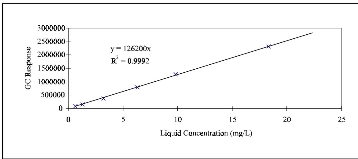
**Figure 3-3. Liquid-phase calibration curve for ethylbenzene.**
