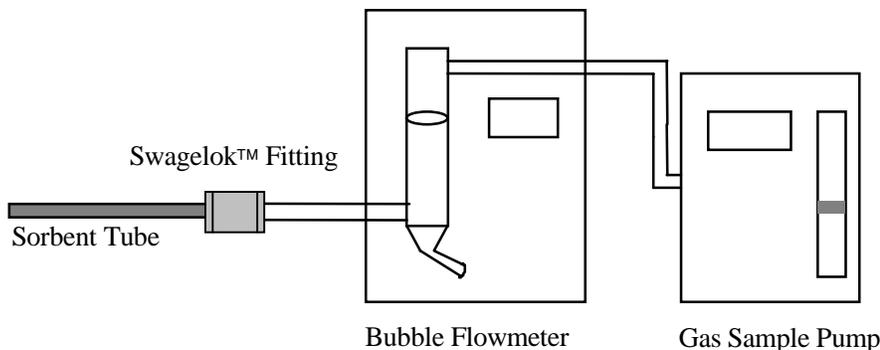
**Figure 3-1. Gas sampling experimental setup.**
