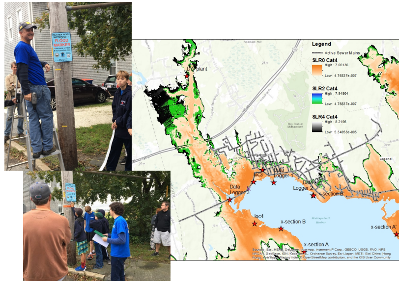
Figure 2. SLOSH modeling results of storm surge inundation for category 4 hurricane and 4-ft sea level rise scenario, with impacts to the wastewater collection and transfer systems. Citizens were engaged in historical flood level identification as a part of the citizen science project.
