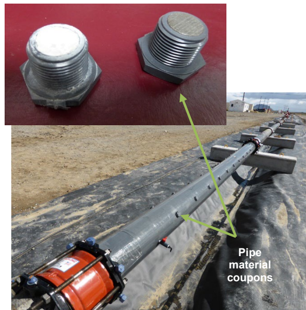
Figure 6: Removable pipe coupon section and images of the coupons.
