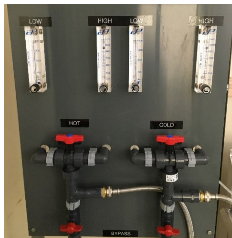
Figure 9: Flow meters downstream from the utility sink used to control flow through the premise plumbing system.
