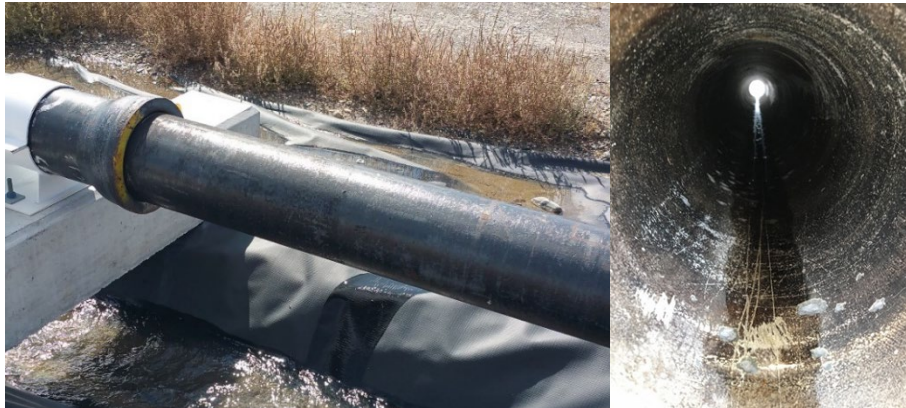
Figure 5: External and internal view of the cement-mortar lined pipe.
