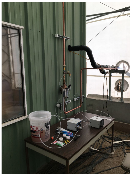
Figure 10: Malathion contamination of the premise plumbing system. Diluted malathion is pumped from a bucket into a flow meter, where it flows into the copper pipe.
