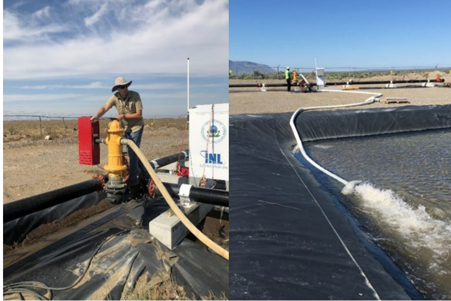
Figure 8: Flushing contaminated water from the WSTB distribution pipe via the downstream fire hydrant. The left image is the fire hydrant with the hose connected, and the hose in the lagoon with sandbags is on the right.
