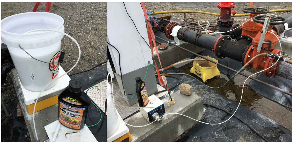
Figure 7: Malathion contaminant injection setup in the 450 ft pipe.
