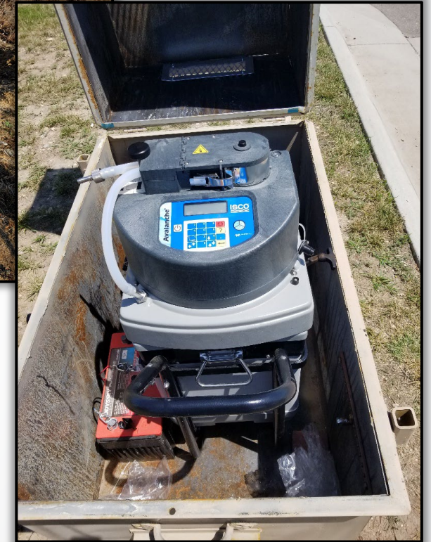
Picture showing the type of runoff sampler to be installed at the MAR site.
