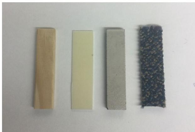
**Figure 2-1. Coupon Types from Left to Right: Pine Wood, ABS Plastic, Ceramic Tile, Carpet.**
