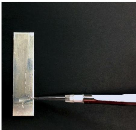
**Figure 2-2. Liquid Inoculation of Coupon Using a Micropipette**
