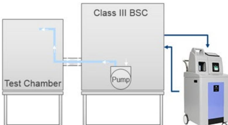
**Figure 2-3. Schematic Diagram of LCHPV Exposure Chamber**
