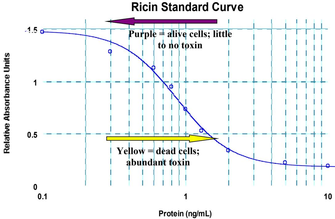
Figure 2-7. Example of Ricin Cytotoxic Profile with Corresponding Absorbance Measured Using a Microplate Reader
