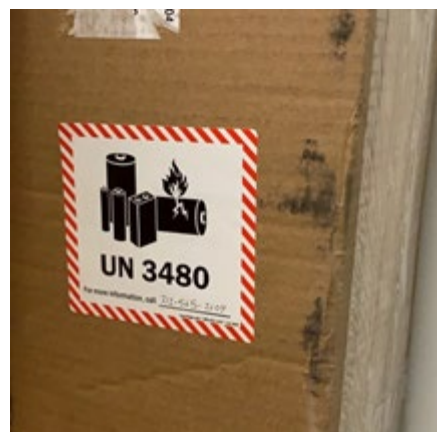
Figure 7. Example of Proper Labeling for a Lithium Battery Shipment
