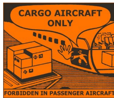
Figure 8. Additional Package Marking for Large Lithium Batteries
