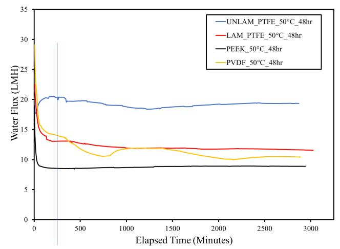
• The water flux stabilizes within ~200 min
