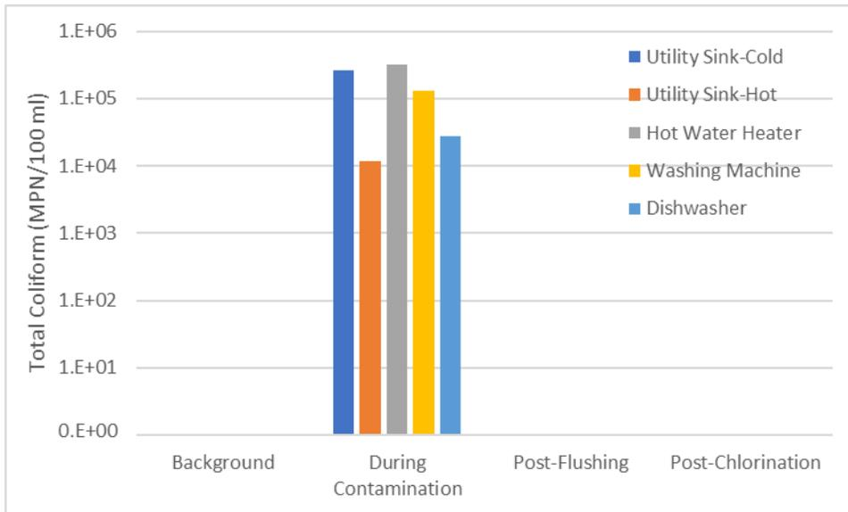
**Figure 17: Total coliform levels in the bulk water phase of the pipes and appliances in the home plumbing system.**
