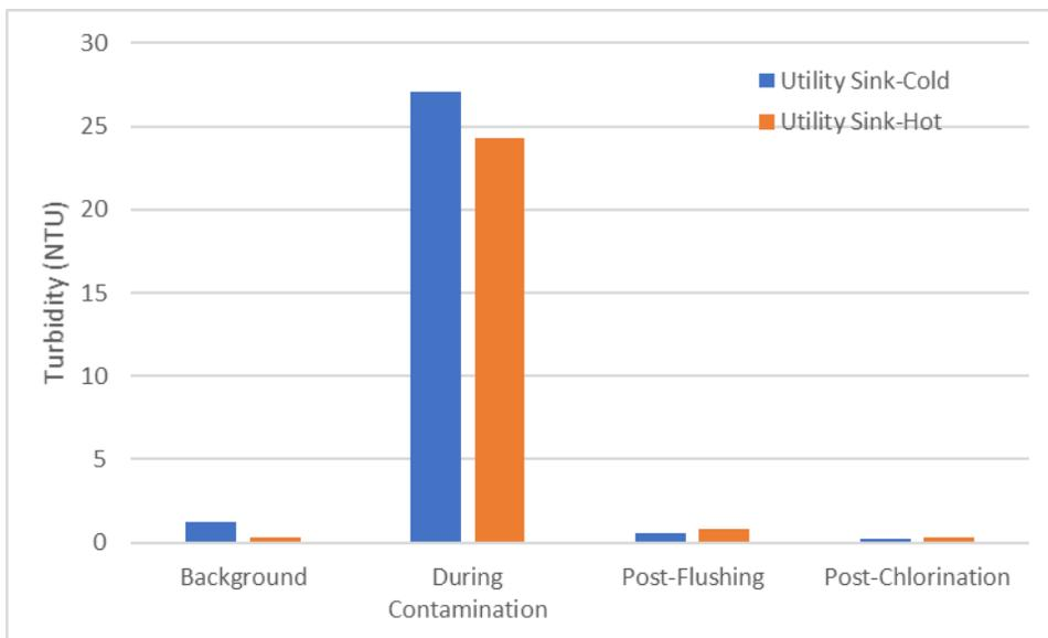
**Figure 21: Turbidity levels at the hot and cold taps in the home plumbing system.**
