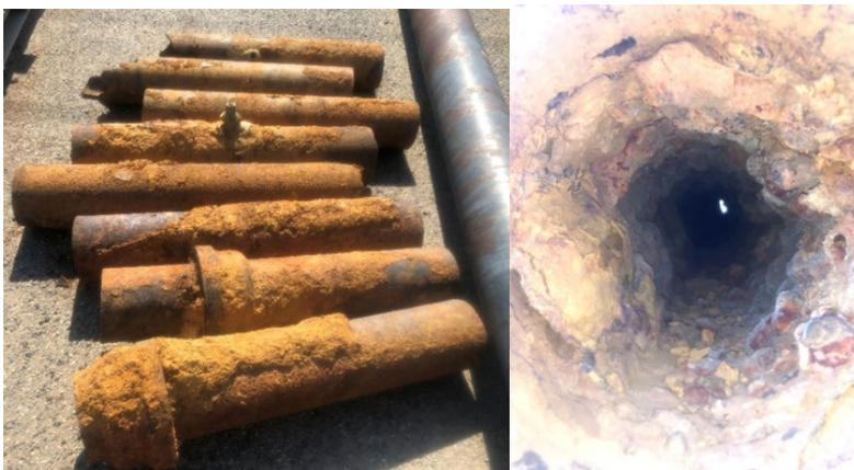
**Figure 7: External (left) and internal (right) view of the cast iron pipe with heavy corrosion (tuberculation) on the interior.**
