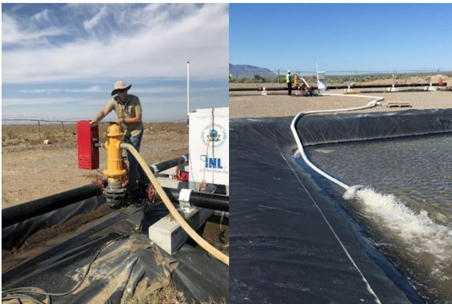
**Figure 10: Flushing contaminated water from the WSTB distribution pipe via the**
