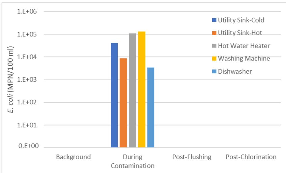
**Figure 18: E. coli levels in the bulk water phase of the pipes and appliances in the home plumbing system.**
