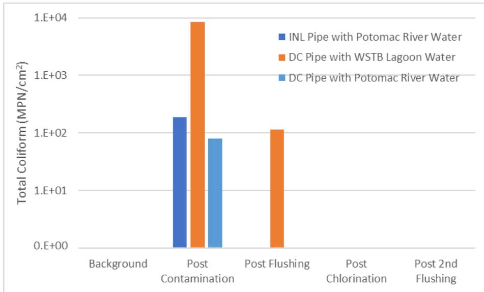
**Figure 24: Total coliform levels on the inner pipe wall of the individual short pipe sections.**
