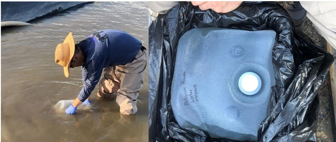
**Figure 8: Mixing *E. coli* into lagoon water (left) and a carboy of Potomac River water (right).**
