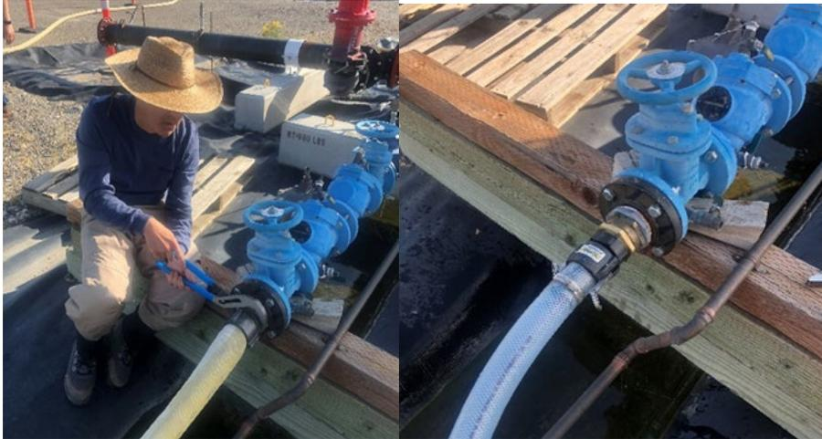
**Figure 9: The setup used to contaminate the WSTB pipe with lagoon water: hose connected to pump in lagoon (top left), hose from lagoon across WSTB site (top right), disconnection of fire hose (bottom left), and connection of lagoon hose (bottom left).**
