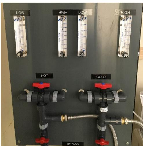
**Figure 12: Flow meters downstream from the utility sink used to control flow through the premise plumbing system.**
