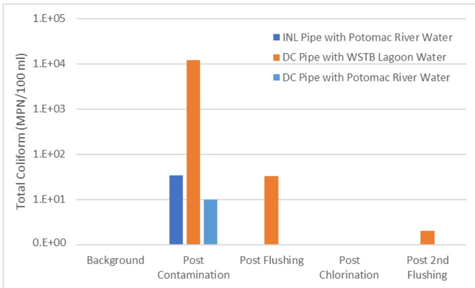
**Figure 23: Total coliform levels in the bulk water phase of the individual short pipe sections.**
