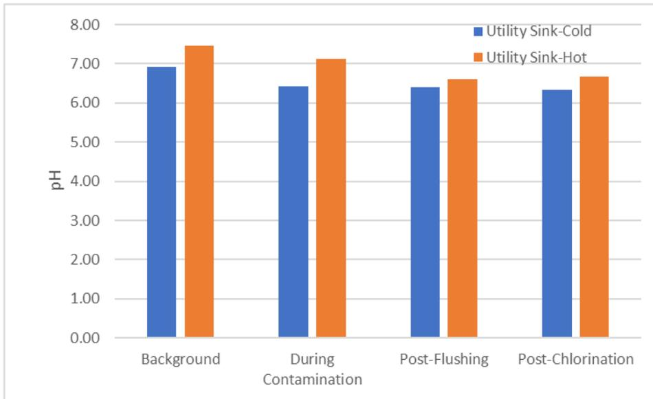
**Figure 20: pH levels at the hot and cold taps in the home plumbing system.**
