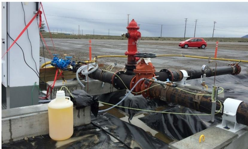
**Figure 11: Example of how chlorine was introduced to WSTB distribution pipe.**
