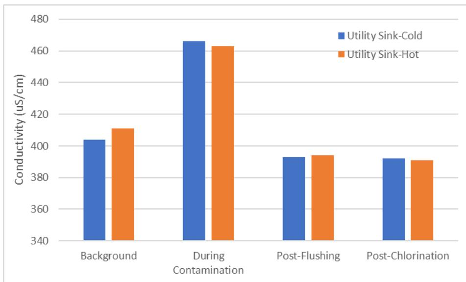
**Figure 22: Conductivity levels at the hot and cold taps in the home plumbing system.**
