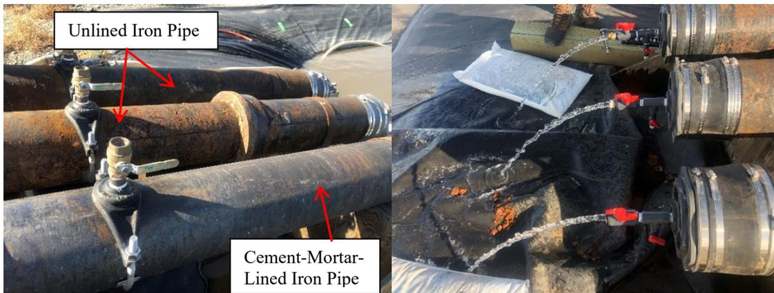
**Figure 4: Individual pipe sections next to the Water Security Test Bed lagoon (left) and the**
