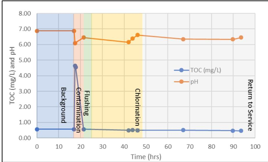
Figure 16: TOC and pH during each stage of the decontamination experiment.
