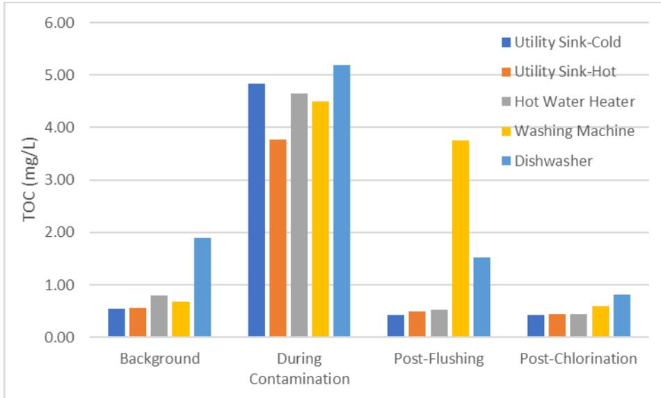
**Figure 19: TOC levels in the bulk water phase of the pipes and appliances in the home plumbing system.**
