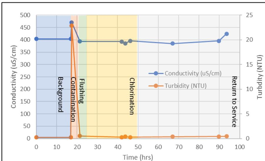
**Figure 15: Conductivity and turbidity measurements during each stage of the**
