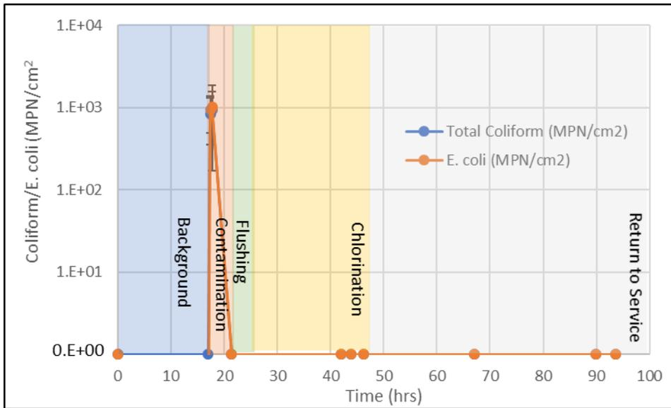
**Figure 14: Contamination and decontamination of coliforms/*E. coli* from the pipe surface of the 450-ft cement-mortar-lined iron distribution pipe.**
