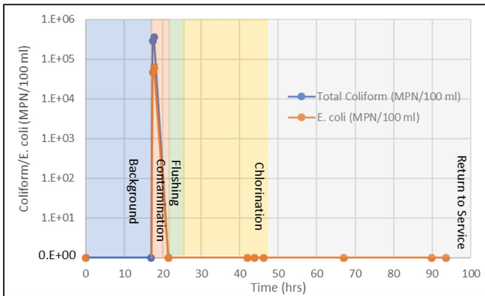
**Figure 13: Contamination and decontamination of coliforms/*E. coli* in the bulk water phase of the 450 ft cement-mortar lined iron distribution pipe.**
