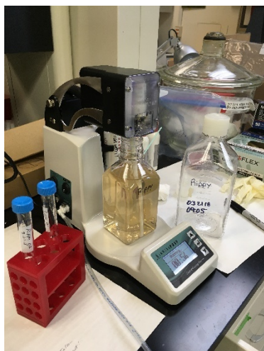
Figure 2. Concentrating water samples using the InnovaPrep instrument.
