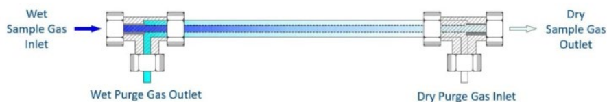
Figure 3. Schematic of Nafion™ tube configured with active purge air for drying of sampled airstream.
