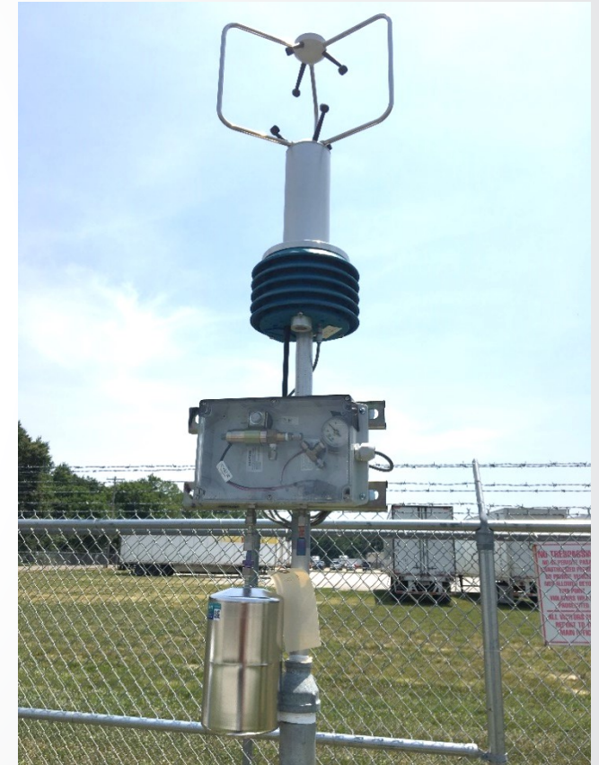
A VOC sensor can be used to trigger a canister sample for more detailed offline analysis
