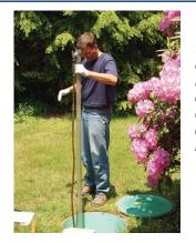
The tool shown is used to measure the depth of sludge and scum layers. If those layers comprise at least 35% of the tank's storage capacity, your tank will need a pump-out.
