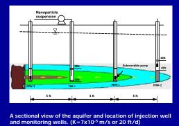
The Nanoparticle Tank and Injection Setup
