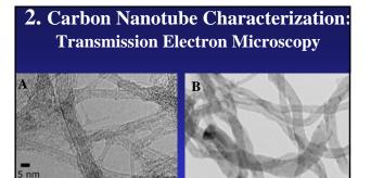
Transmission electron micrographs of (A) single-walled at 250kx magnification and (B) multi-walled carbon nanotubes at 100kx magnification.
