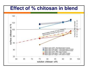
Test Surface Properties -Electrospun chitosan fibers
