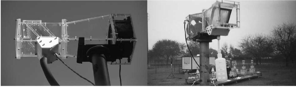
Fig. 2. The Caltech Heated Rod Cloudwater Collector (CHRCC) (left) and the Caltech Active Strand Cloudwater Collector version 2 (CASCC2) (right).
