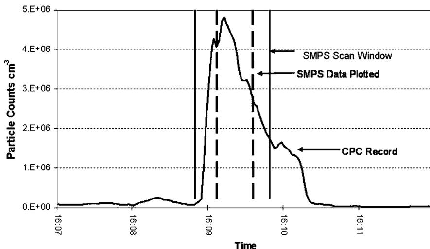
Fig. 5. Particle counts recorded by TSI Model 3022a while an aircraft prepared for takeoff at site D. SMPS scan performed during period enclosed by solid vertical lines, data displayed in Fig. 7 obtained from constrained file assembled from time period between dashed lines.
