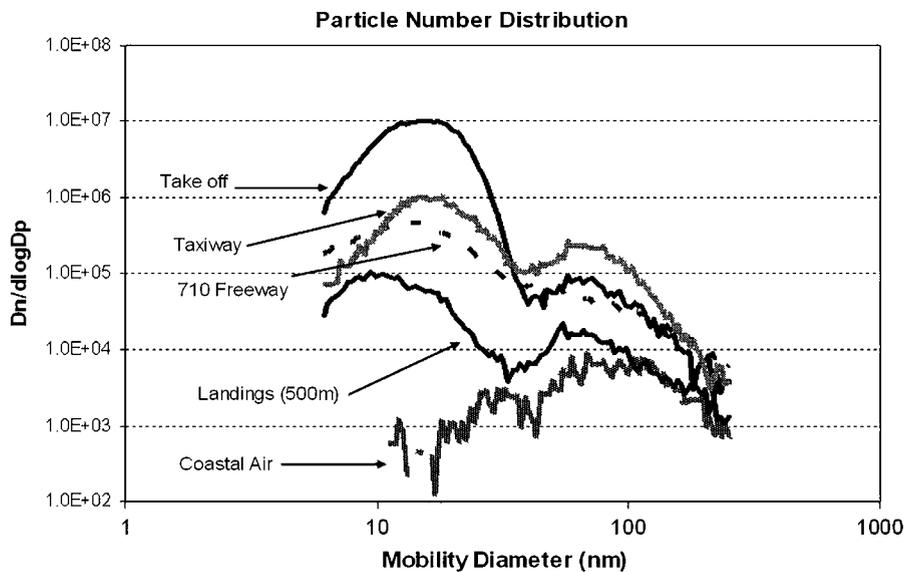
Fig. 8. Display of particle size distribution of clean coastal air, at various locations near LAX, on a segment of the 710 Freeway. Bimodal distributions are apparent in areas with combustion particles.
