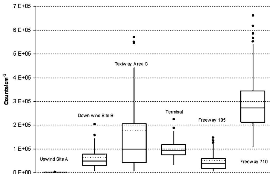
Fig. 3. Comparison of particle counts at various locations near LAX and on Freeway 710, a roadway with a large proportion of diesel trucks.
