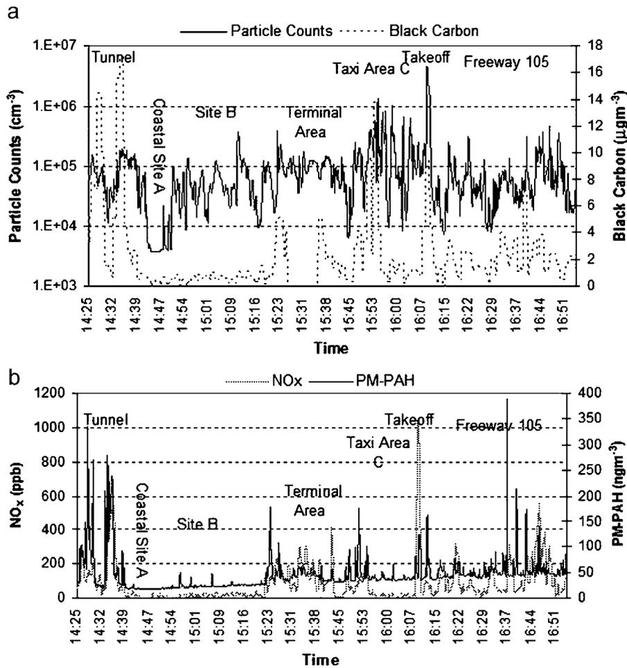
Fig. 2. Time series display of observations in and around LAX: (a) displays data for particle counts and BC, while (b) displays PM-PAH and NO<sub>x</sub>. Note that particle counts are displayed on a log scale.
