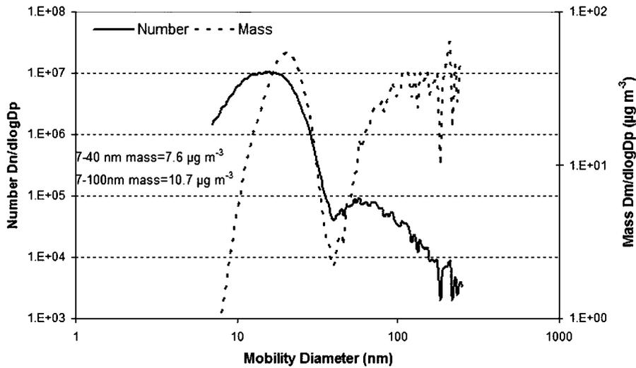
Fig. 7. Particle number and mass distribution observation made during the takeoff of a jet aircraft at site D. Mass estimates are shown for first peak (7–40 nm) and for UFP size range (7–100 nm) with estimated particle density of  $1.2 \text{ g cm}^{-3}$ .
