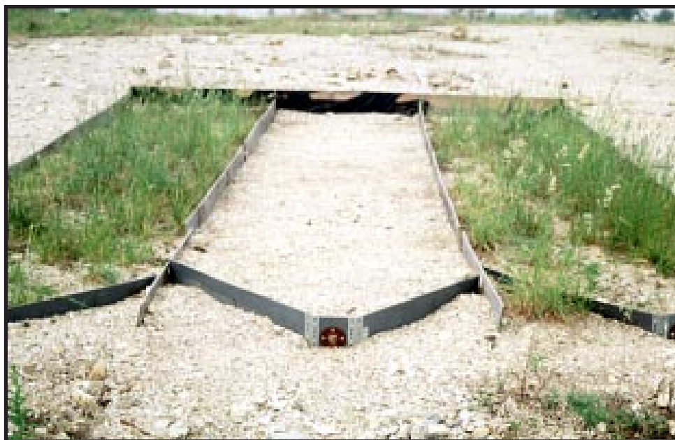
Figure 2. Test plots for evaluating revegetation of chat material in Galena, Kansas. Here, tall fescue is being grown as a way of reducing sediment runoff and the spread of heavy metal pollution. The bare center plot is a control in which fescue was not planted.
