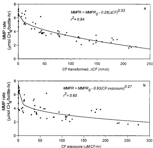
FIGURE 3. MMP rates vs (a) mass of CF transformed and (b) CF exposure from the two-phase, CF biotransformation toxicity experiment. The equation of the best-fit nonlinear equation is shown.
