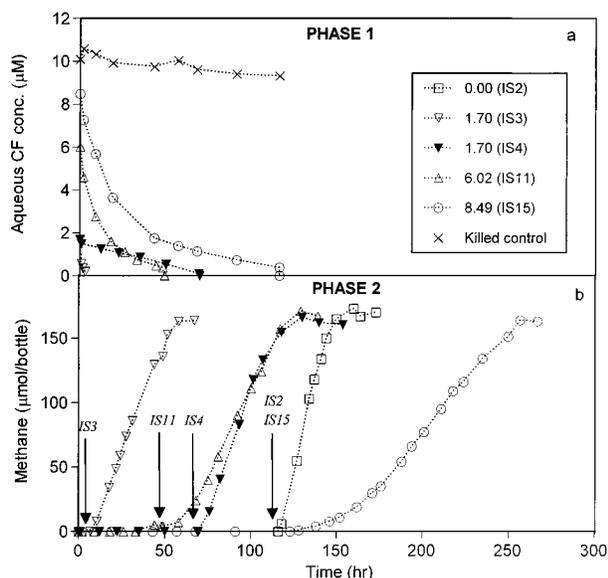
FIGURE 2. CF transformation (a) and methane production (b) in selected incubation sets (IS) from the two-phase, CF biotransformation toxicity experiment. All incubations except those indicated by filled symbols (IS4) received acetic acid in phase 1. Mean values of quadruplicate bottles are shown. Arrows indicate when incubations were sparged with  $N_2/CO_2$  gas. Legend gives initial CF concentration ( $\mu$ M CF) and incubation set number. See Table 1 for the results of all incubation sets.
