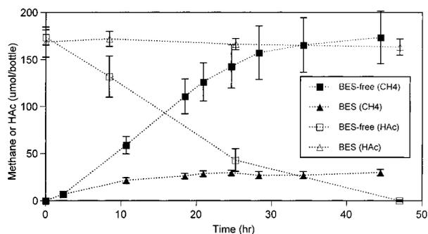
FIGURE 1. Inhibition of aceticlastic methanogenesis by 50 mM BES, a specific methanogenic inhibitor. Thirty-eight-milliliter serum bottles containing 25 mL of cell suspension were amended with 10  $\mu$ L of acetic acid. Mean values of duplicate bottles are shown. Error bars show  $\pm 1$  SD.
