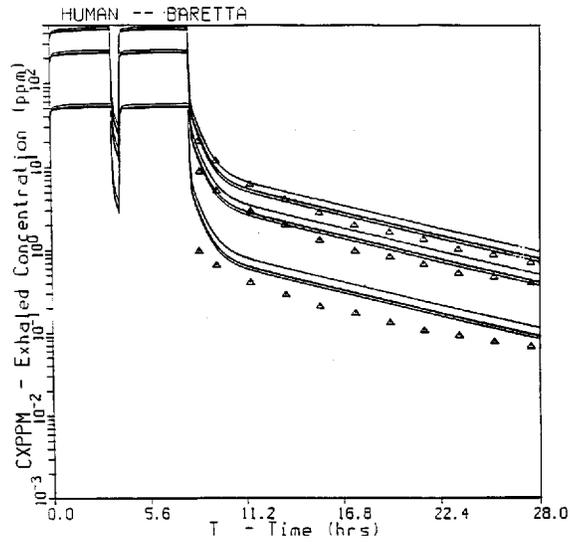
**Figure B-7. Model predictions (lines) and experimental data (symbols) for the exhaled air concentration following inhalation exposure of human subjects for 8 hr (with a 30-min break for lunch) to a constant concentration of (top to bottom) 492, 261, and 59 ppm VC (Baretta et al., 1969). At each concentration the three lines show the model predictions for (top to bottom) VMAX1C = 0, 4, and 8. The rest of the model parameters are those shown for the human in Table A-1.**
