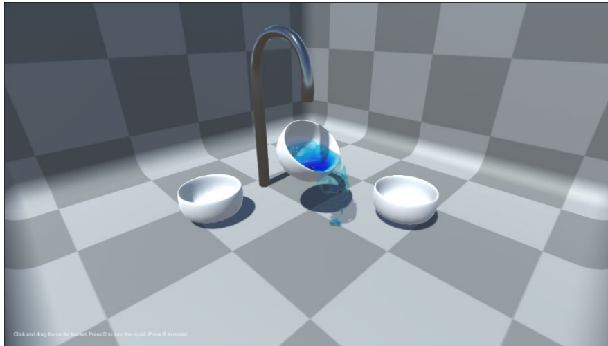
Figure 2. SPH Fluid Simulation of Water Flowing from a Faucet to a Bowl That Can Be Tilted
