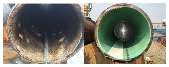
Figure 7: Pipes lined with Oceanit DragX (left) and CIPP (right).
