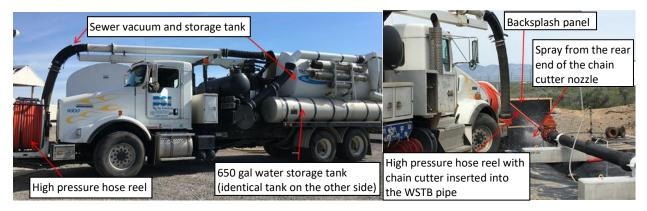
Figure 5: A combination truck (left), and a nozzle being inserted into the Water Security Test Bed pipe for decontamination (right).
