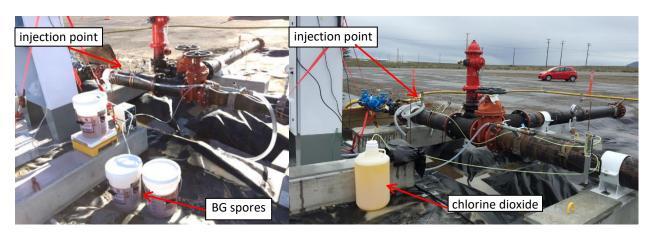
Figure 2: Injection of *Bacillus* (BG) spores (left) and chlorine dioxide (right) into the pipe.
