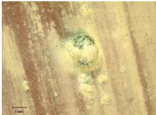
Pitting is a localized acceleration of corrosion that results in the thinning of the pipe wall in the effected area.
