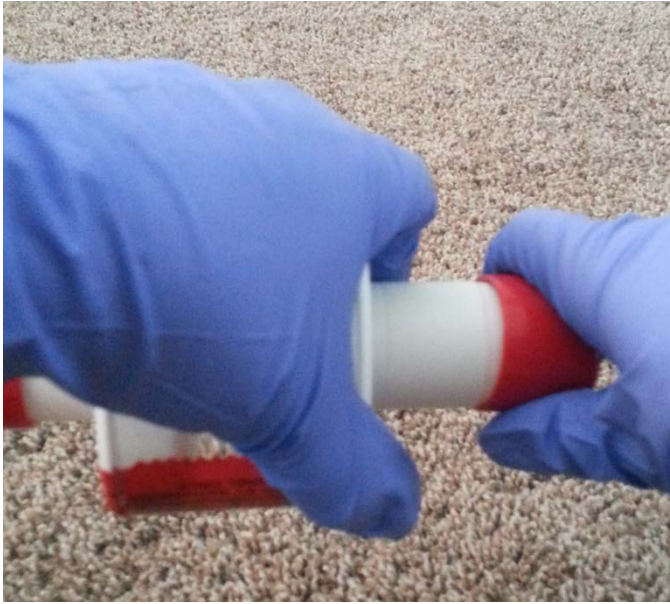
Figure 5. Proper hand placement to remove red end caps from forensic vacuum filter cassette.
