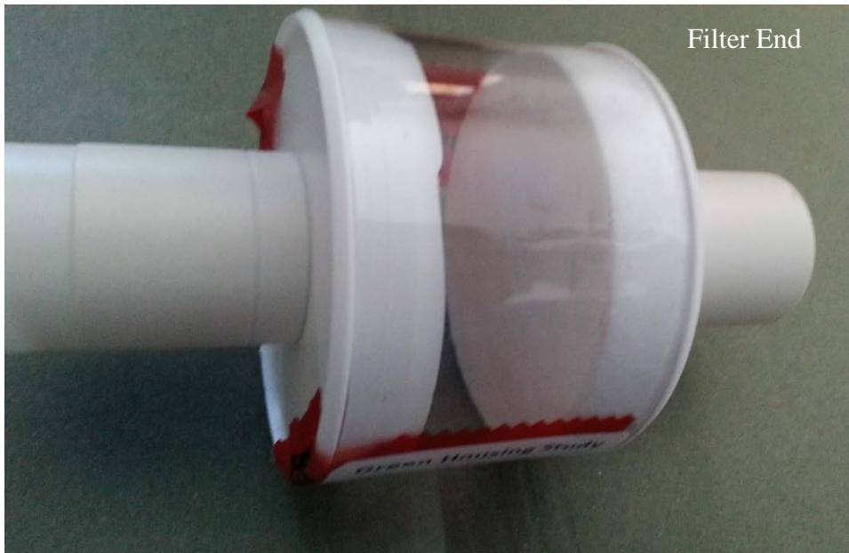
Figure 7. Filter end of the forensic vacuum filter cassette (without the black gasket).
