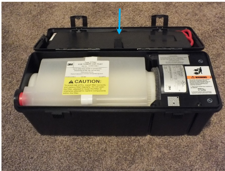
Figure 2. Open 3M Trace Evidence Collection vacuum box.
