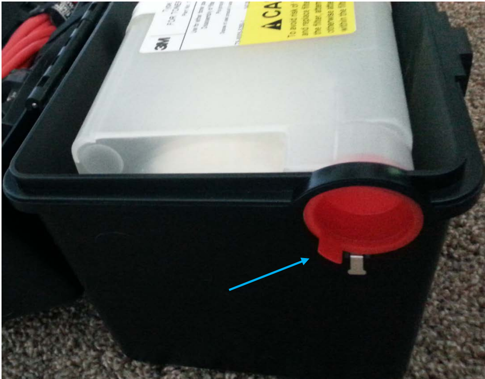
Figure 6. Left side of 3M Forensics vacuum showing cap covering vacuum inlet.
