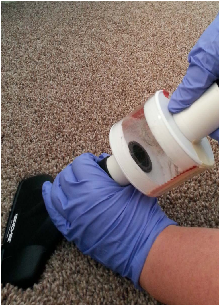
Figure 10. Proper grasp of forensic vacuum filter nozzle and cassette for sampling.
