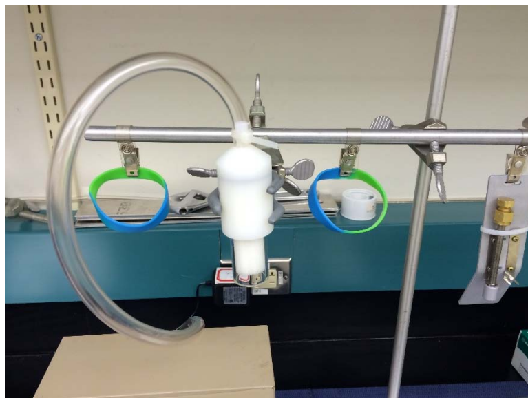
Figure 1. Passive samplers clipped onto the sampling stand.
