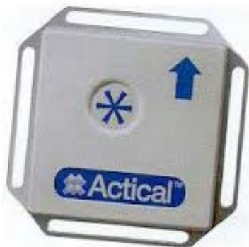
Figure 10. Front of Actical™ device showing arrow that should point up towards the participant's head after correct deployment.
