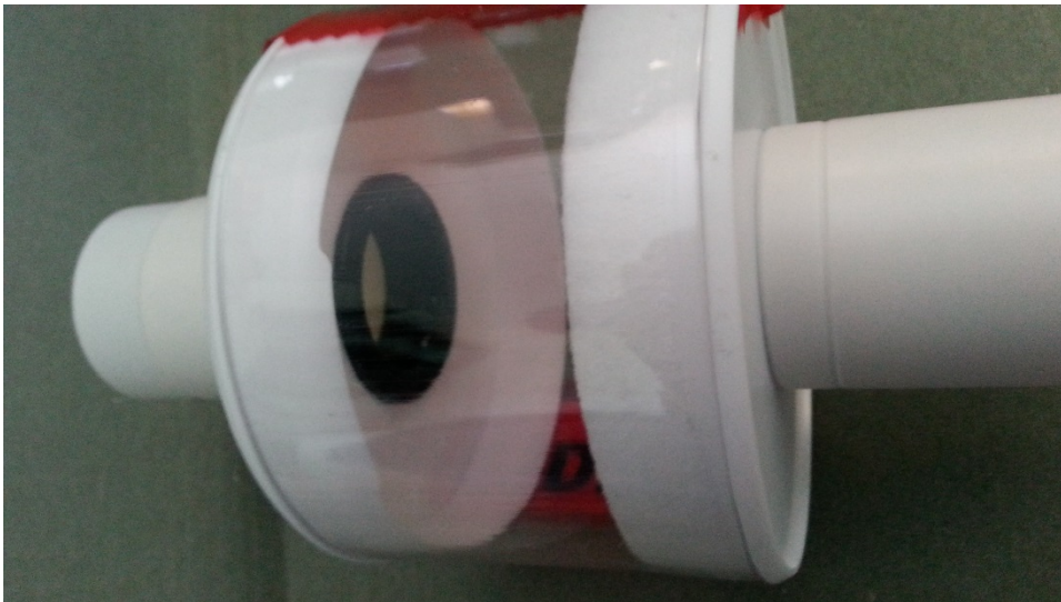
Figure 8. Open/non-filter end of the forensic vacuum filter cassette (with black gasket).
