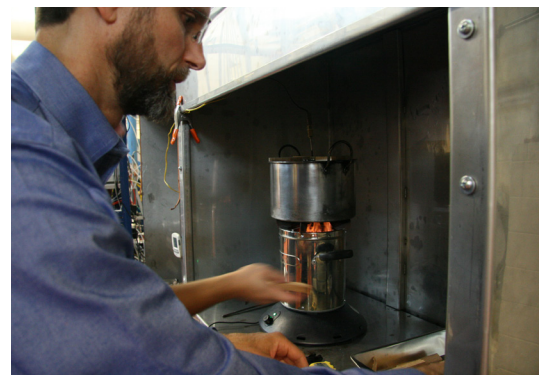
Above, Jim Jetter, EPA, tests a wood-fueled forced-draft stove for air pollutant emissions.
