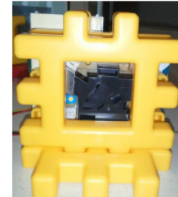
Figure 2. Sensor kit components assembled using a children's building toy pieces and velcro
