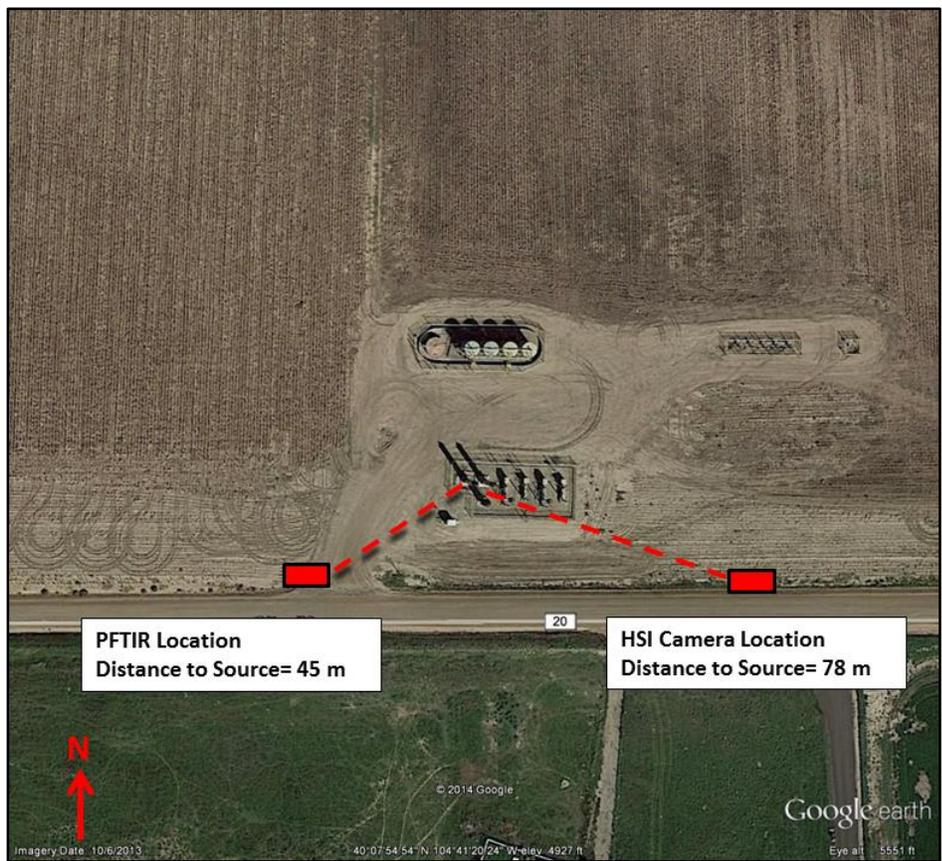
The PFTIR detected emissions of several hydrocarbons from the stack. A summary of path-integrated concentrations determined from data collected with the PFTIR is presented in Table 2.
