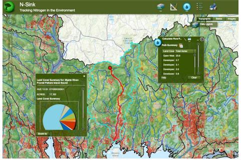
This screen capture shows calculation of a flow path from source to watershed outlet (red line). A web-based beta version of N-Sink is available at http://clear.uconn.edu/projects/nsink.
