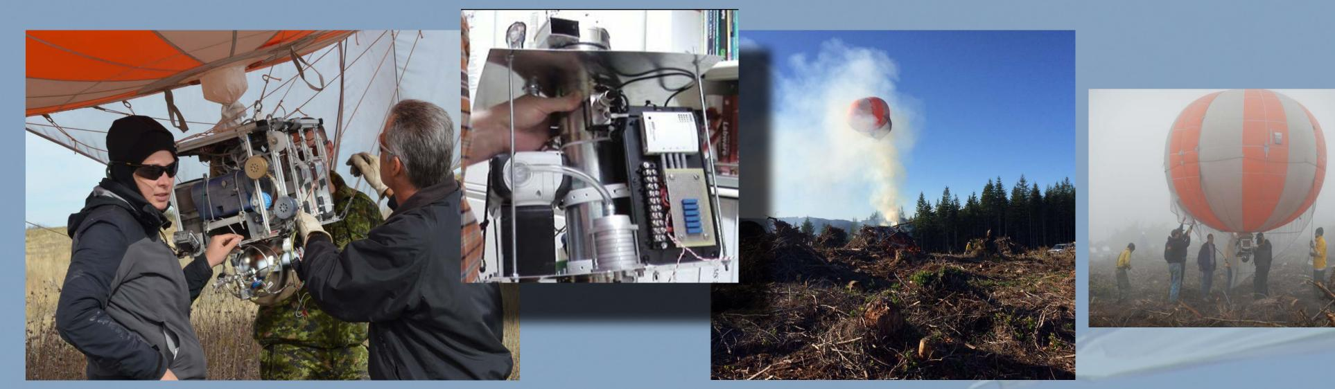
The aerial sampler "Flyer" is used for open burn measurements in the field at prescribed altitudes.
