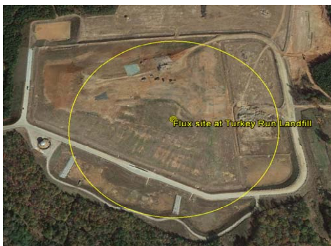
Fig. 1. A Google Earth image showing the flux footprint with a radius of 200 m at Turkey Run Landfill
