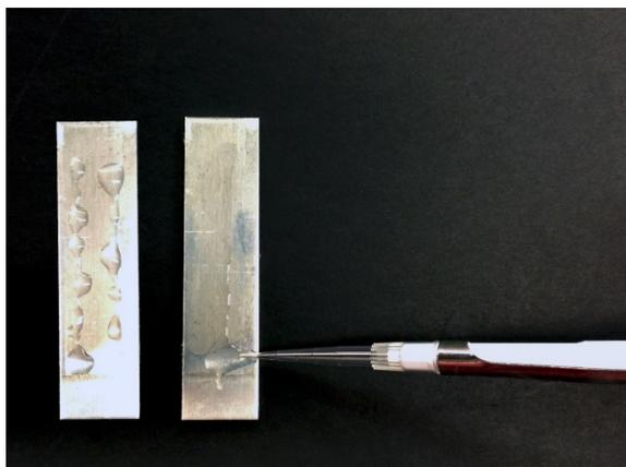
**Figure 3-2. Liquid Inoculation of Coupon Using a Micropipette**
