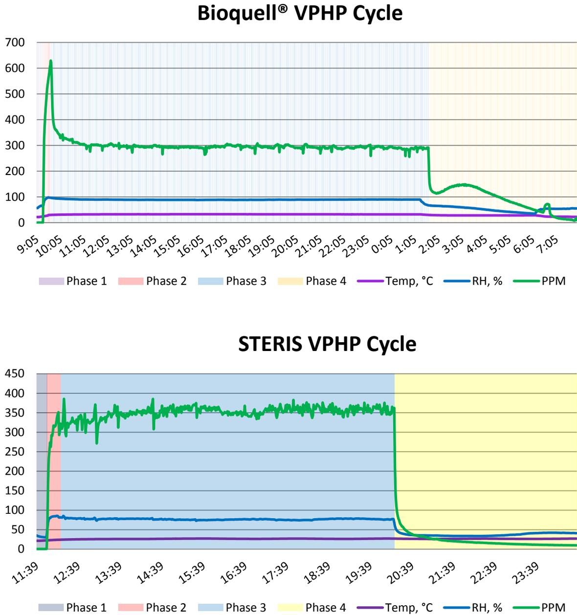
**Figure 3-4. Representative Graph of Bioquell and STERIS Decontamination Cycles**
