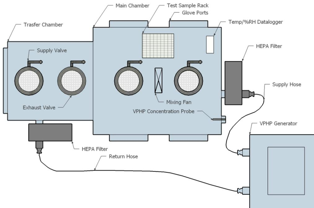
**Figure 3-3. Aerial Schematic of VPHP Test Chamber and Attached Fumigant Generator**
