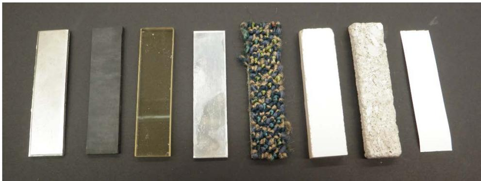
**Figure 3-1. Coupon Types from Left to Right: Aluminum, Neoprene Rubber, Optically Clear Acrylic, Stainless Steel, Industrial Carpet, Ceramic Tile, Unpainted Concrete, and Paper**
