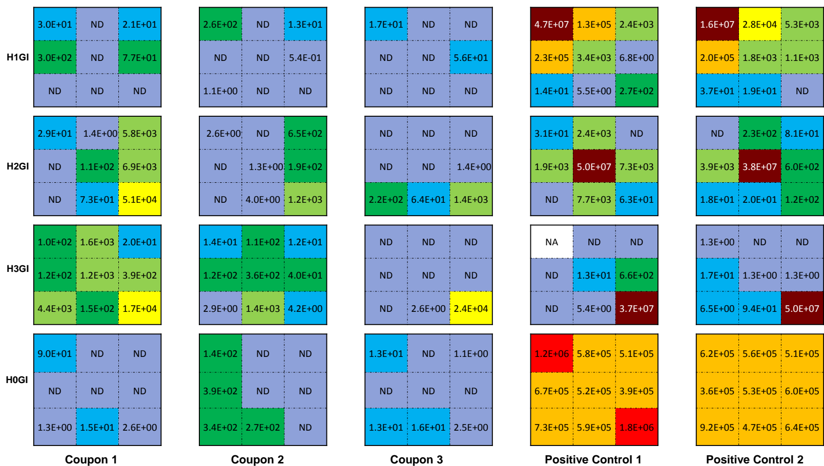
Figure 4-8. Spatial Post-Decontamination Residual Spore Concentration Using Hype-Wipe® Bleach Towelette /Glass Material at Different Inoculation Locations.
