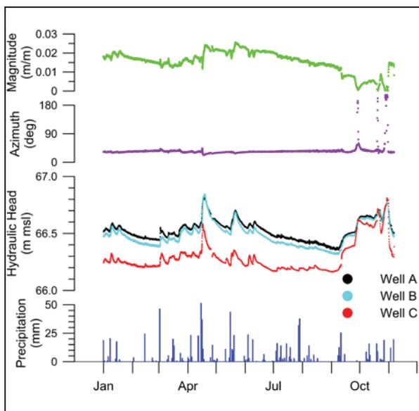
Figure 13. Hydraulic heads measured using pressure transducers in three wells and the resulting magnitude and direction (azimuth) of the hydraulic gradient measured in degrees from North. Precipitation data was obtained from a nearby meteorological station.
