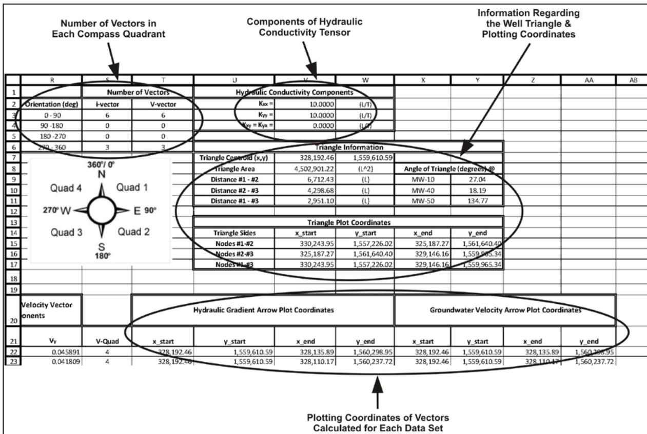
Figure 4. Screen capture from the 3PE spreadsheet depicting results describing the orientations of the vectors, the triangle of wells used to calculate hydraulic gradients, the components of the horizontal hydraulic conductivity tensor, and the vector plotting coordinates calculated for each data set.
