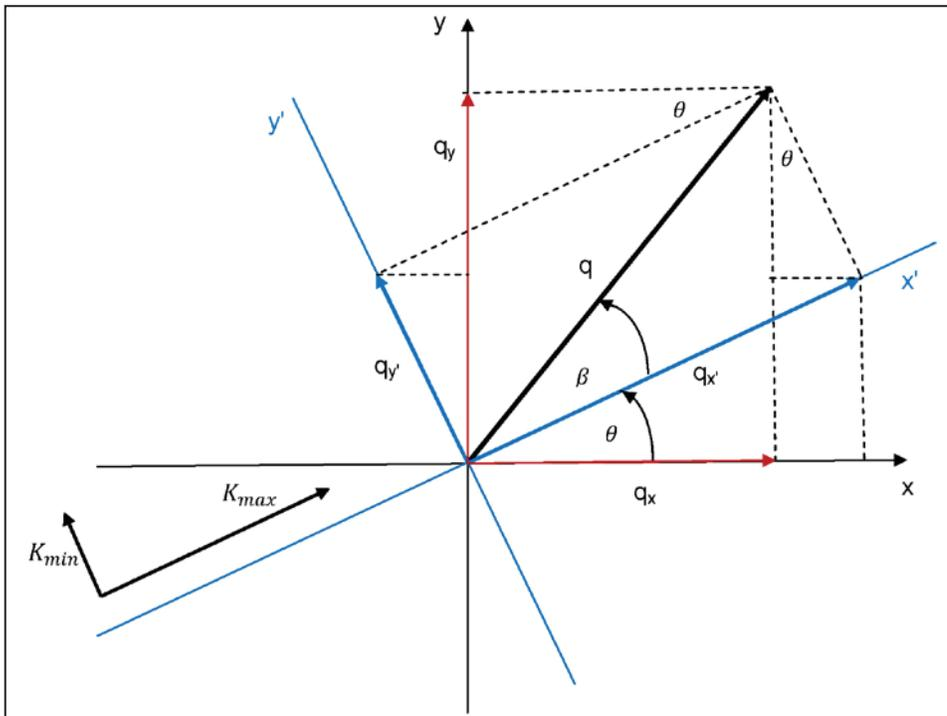
Figure A-3. Representation of the rotation of the coordinate system so that the principal directions of anisotropy,  $K_{max}$  and  $K_{min}$ , correspond with the coordinate system  $x', y'$ , respectively.
