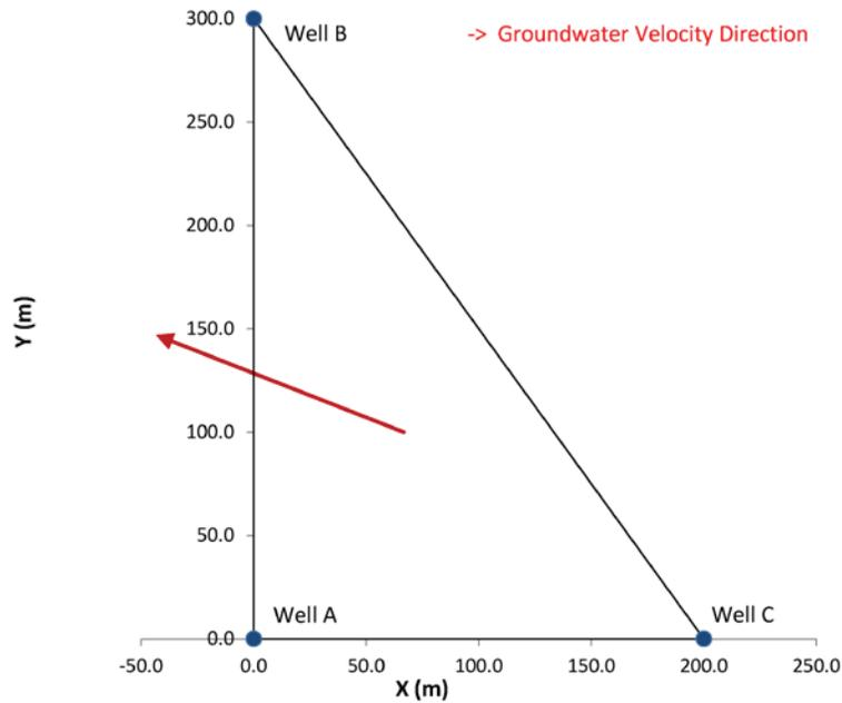
The orientation of the groundwater flow velocity vector calculated by 3PE is 293 degrees (23 degrees clockwise from the negative x-axis), which is identical to the published answer.
