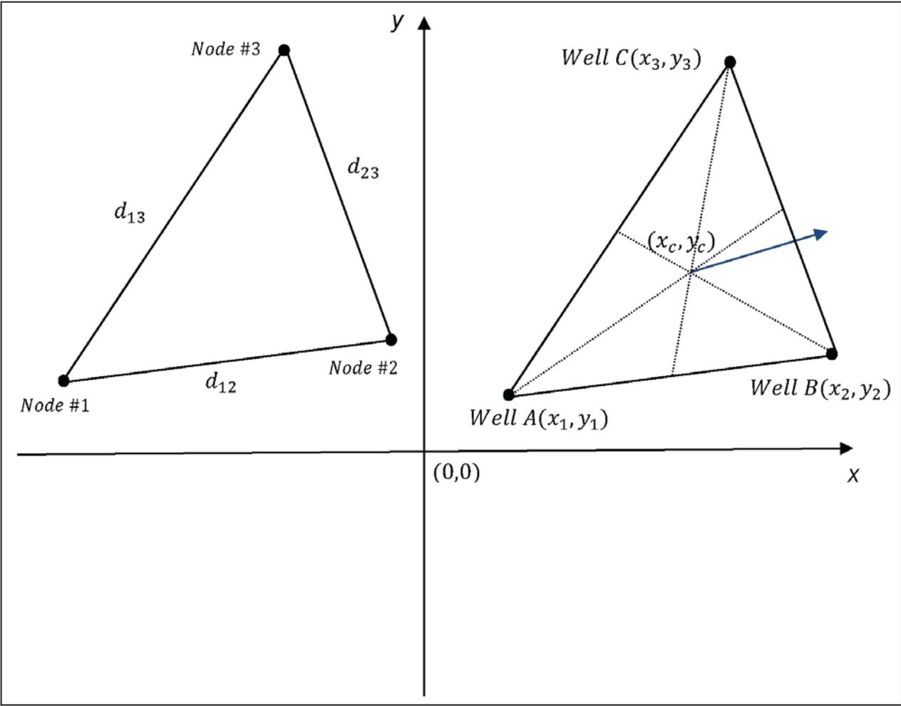
Figure A-1. Representation of the wells in a two-dimensional Cartesian system as implemented in the 3PE spreadsheet. Terminology used to designate the sides and vertices of the triangle (well locations) is depicted in the left triangle. The well coordinate convention and location of the centroid of the triangle are depicted in the triangle on the right.
