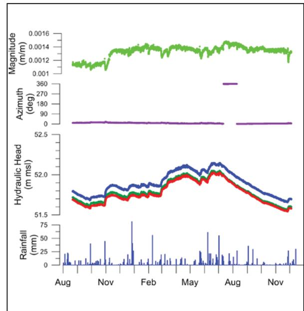
Figure 15. Hydraulic heads measured using pressure transducers in three wells and the resulting magnitude and direction (azimuth) of the hydraulic gradient measured in degrees from North. Precipitation data were obtained from a local meteorological station.
