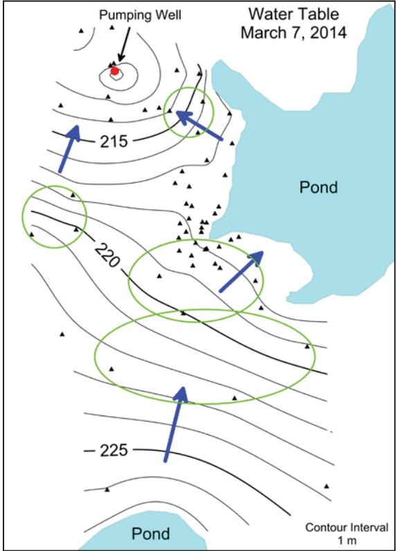
Figure 6. Example potentiometric surface map interpreted from hydraulic head data measured in multiple wells (black triangles). In general, groundwater flows from areas where it enters the aquifer to areas where it leaves the aquifer. Blue arrows depict groundwater flow directions indicated by hydraulic gradients. Green circles and ellipses highlight examples of areas where the water table is sufficiently planar and wells exist for analysis of hydraulic gradients using three-point methods.
