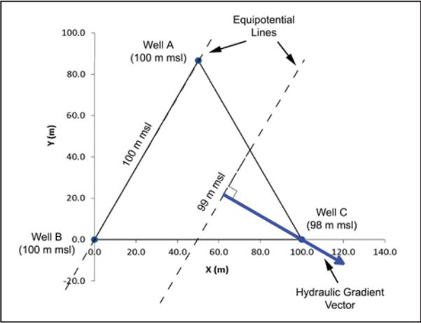
Figure 5. Calculation of hydraulic gradient vector using hydraulic head data from three locations (Wells A, B, and C). The hydraulic gradient vector, calculated graphically using the methods of Heath (1983) in this case, is perpendicular to contours of equal hydraulic head (equipotential lines) and is the direction of groundwater flow in an isotropic setting.
