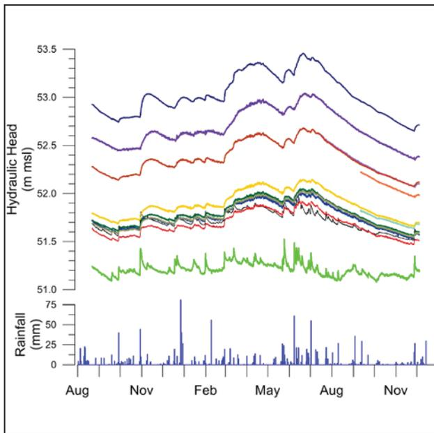
Figure 14. Hydrographs of hydraulic head in monitoring wells and precipitation measured at a local meteorological station.
