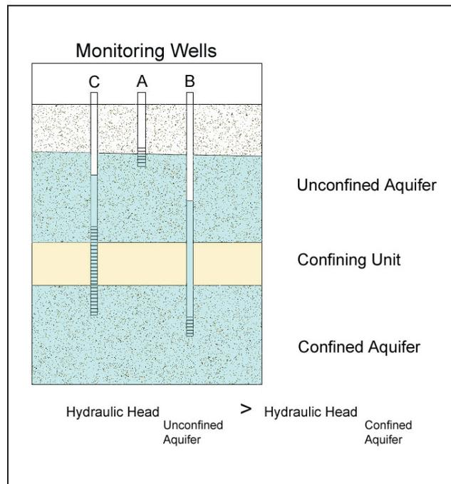
Figure 8. Groundwater elevations in three adjacent wells (A, B, and C) screened at different depths. In this case, Well A is screened across the water table in an unconfined aquifer, Well B is screened in a deeper confined aquifer, and Well C is screened in both aquifers. Differences in hydraulic head in the two aquifers result in significant differences in the groundwater elevations measured in the wells.
