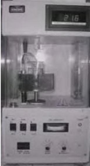
**Figure 12** Digital tensiometer.
