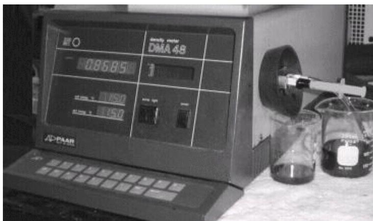
**Figure 4** Digital densitometer taking a reading.
