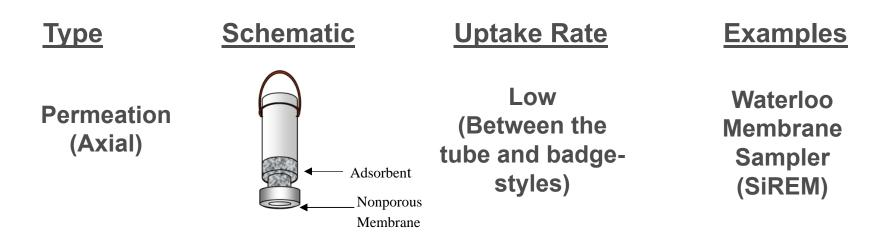
Permeation Design: VOCs dissolve in and diffuse through a nonporous, hydrophobic membrane.
