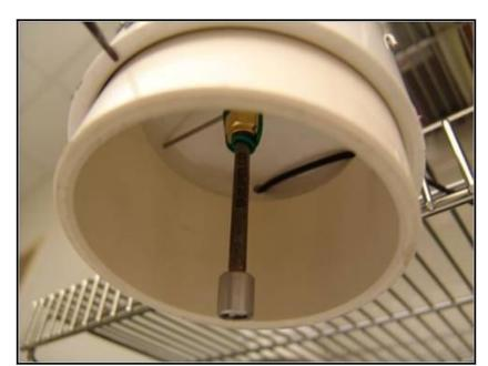
Passive diffusive tube samplers provide a low cost, easy-todeploy way of determining time-averaged fenceline concentrations for many species. The samplers are hung under protective hoods around a facility and are replaced every 2 weeks. Passive samplers provide a useful screening tool to determine areas that may need further LDAR investigation.
