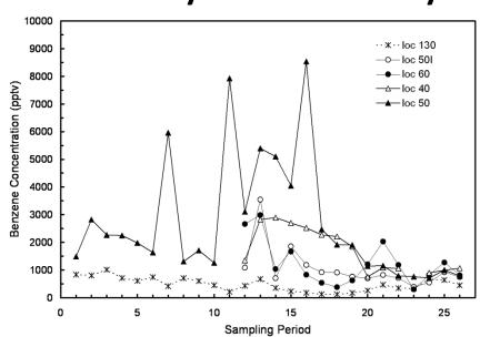
Two-week time-averaged benzene results taken over a one year period at upwind (loc 130) and downwind locations on a refinery fenceline. With steady wind conditions, passive samplers can identify areas for targeted LDAR investigations with more detailed measurements.<sup>1</sup>
