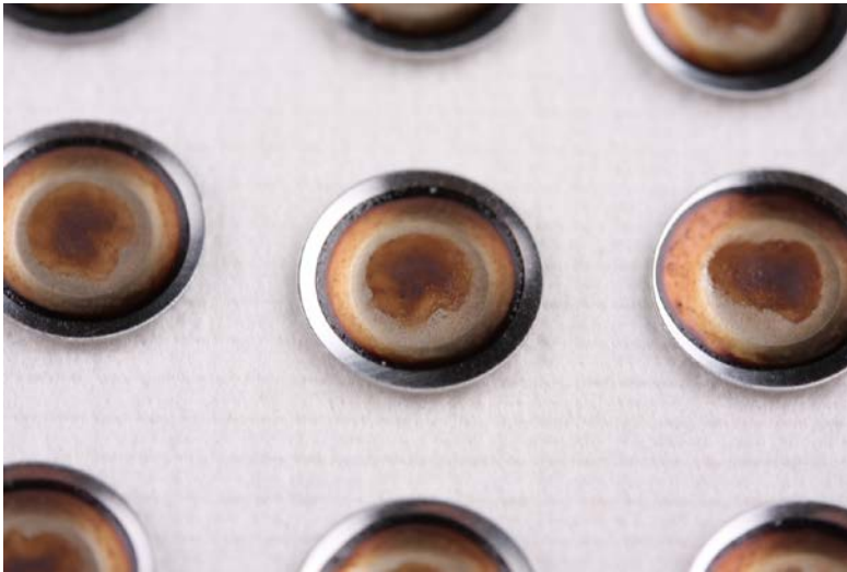
Figure 2-1. Stainless Steel Carrier with Burden and Inoculum
