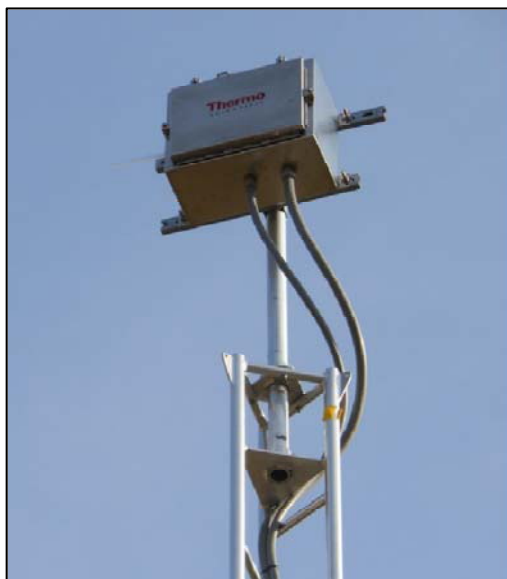
Figure 7. NO y Converter at 10 meters
